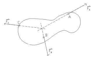
• the lines of action of all three forces must intersect at a point (necessary to satisfy  $\sum \vec{M} = 0$ )
