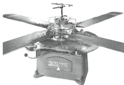
Figure 15.4 Aircraft propeller assembly balancer. (Courtesy of Schenck Ro Tec Corporation, Auburn Hills, MI.)
