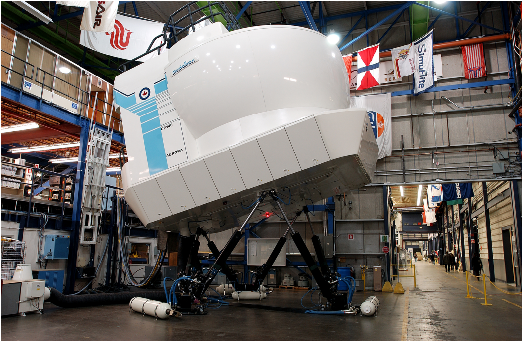
Figure 1.1: CAE's version of a Gough-Stewart motion platform for a flight simulator [3].
