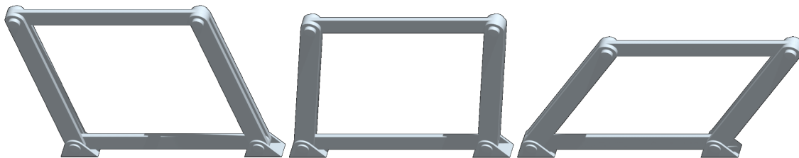
Figure 2.5: 2D Flexible Structure: This 2D structure has one degree of freedom. It can have infinitely many configurations and is therefore non-rigid or flexible [22].
