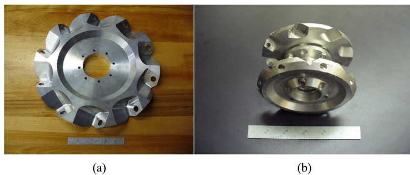
Figure 7 (a) Atlas active wheel hub; (b) Atlas passive wheel hub assembly (see online version for colours)
