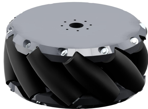
Figure 3. Driving mecanum wheel design.
