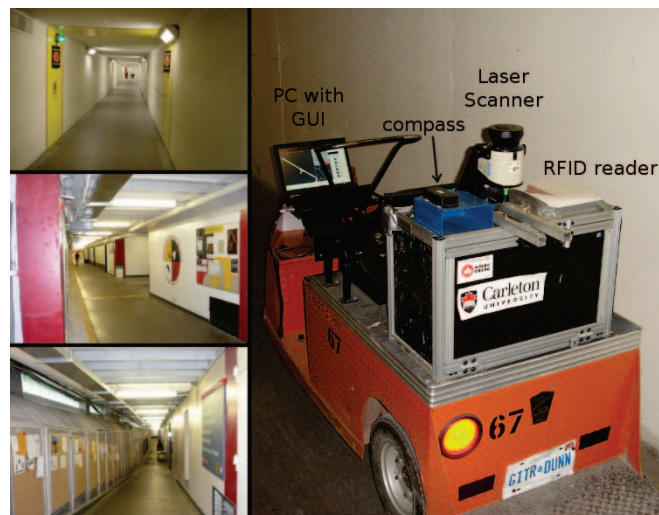
Fig. 3. CU underground tunnels and sensor equipped vehicle.
