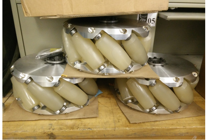
Figure 6. Active mecanum wheels.
