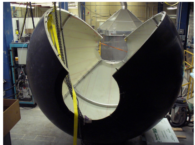
Figure 4. Atlas full-scale internal sphere structure.
