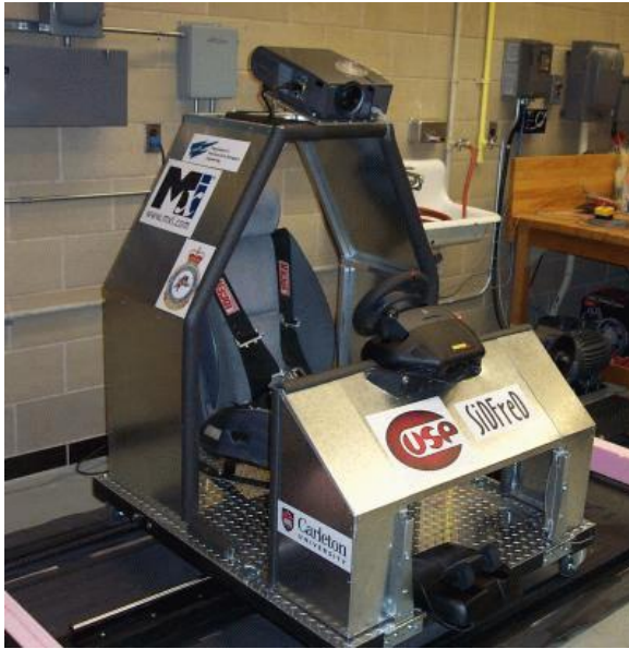
Figure 8: SIDFreD cockpit and translational platform
