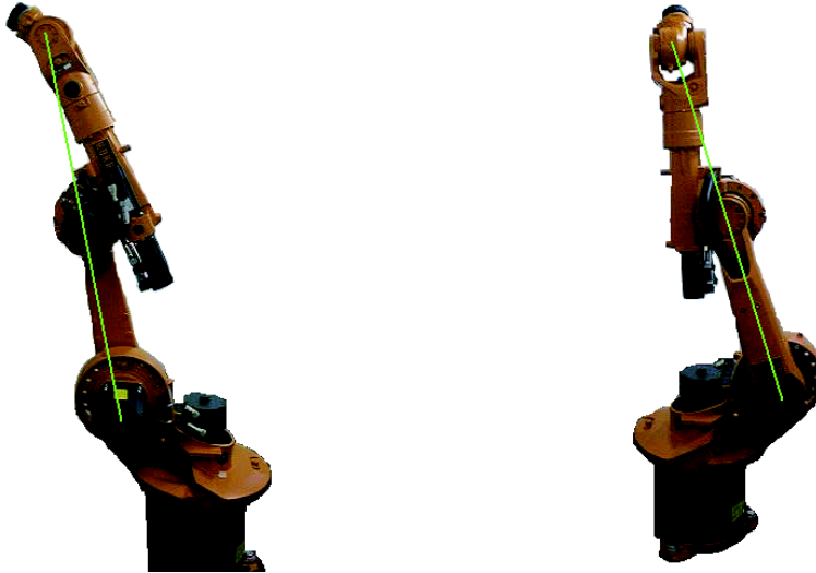
Figure 4: Two KUKA KR-15/2 elbow singular configurations.
