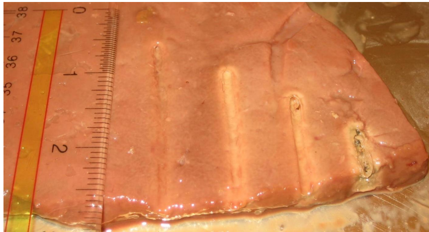
Figure 4.4: Liver cauterization experimental results for varying cauterization probe insertion lengths.
