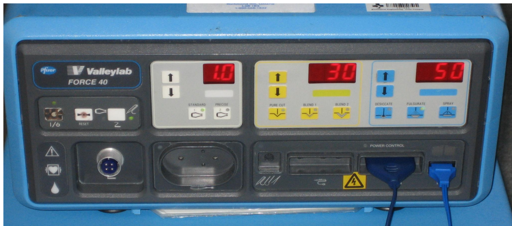
Figure 4.5: Valleylab ESU displaying coagulation power setting of 30 watts , as seen in central display surrounded by yellow buttons.
