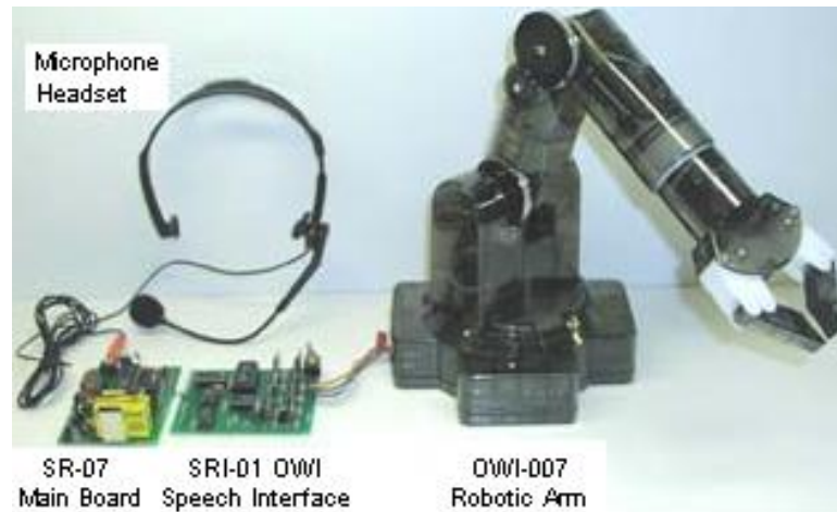
Figure 4.7: Speech Controlled Robotic Arm kit [45], including headset, voice recognition hardware, electrical activation hardware and robotic arm manipulator.
