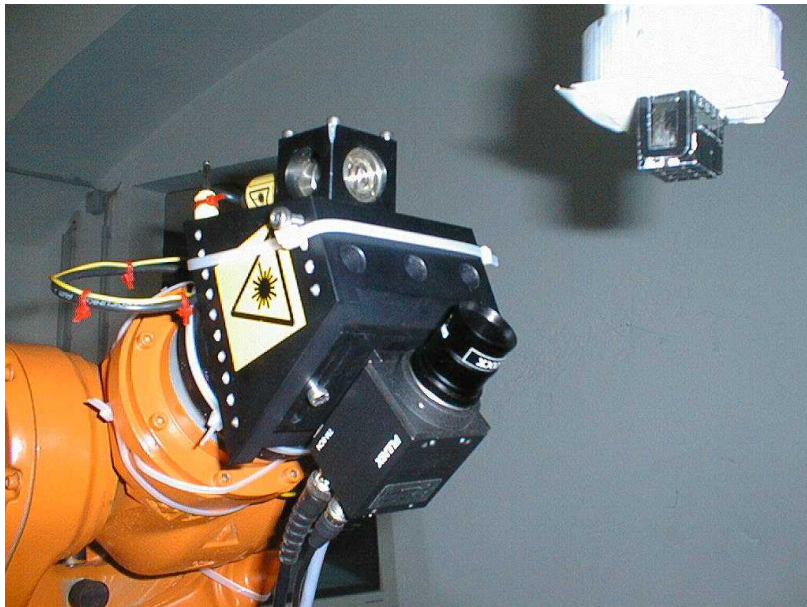
Figure 2.2: Measurement head mounted to KUKA KR-15/2.
