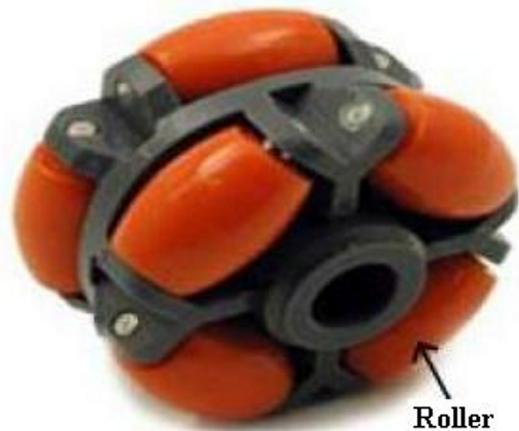
Fig. 4 A dual-race omnidirectional wheel
