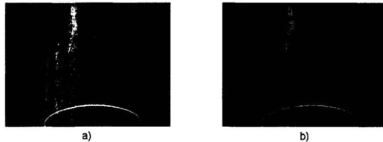
Figure 5.3: Images demonstrating background elimination, (a) before and (b) after the algorithm is applied.
