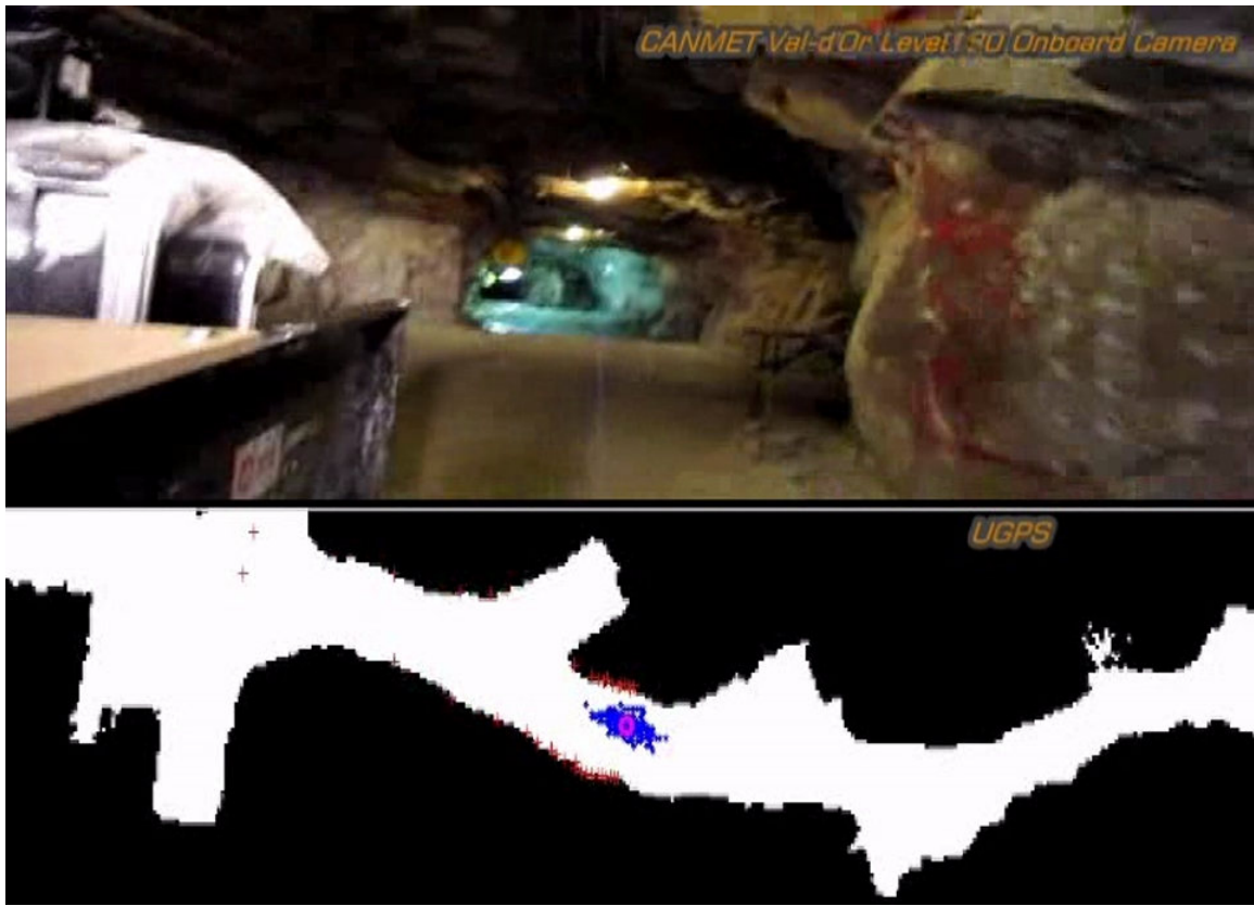
Figure 4.7: Screen shot from offline particle filter localization using data from CANMET Experimental Mine. Rear-view on board camera synchronized with particle filter estimated location.
