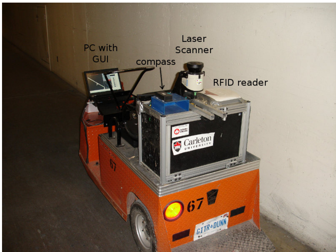
Figure 4.1: Taylor-Dunn SS-534 vehicle with sensors in the CU tunnel network.
