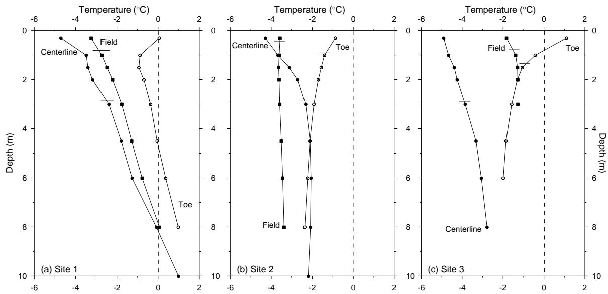
Figure 7. Annual mean temperature profiles from sites 1 – 3 for 1 Mar. 2014 – 28 Feb. 2015. Thaw depths are indicated by a horizontal line at each site. Maximum temperatures were  $> 0^{\circ}\text{C}$  throughout the profile at the toe location of site 1.
