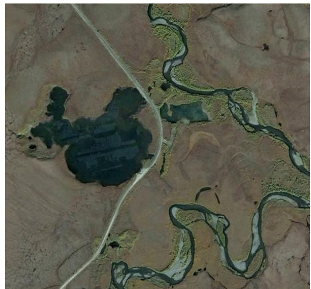
Figure 8. Thermokarst expansion of Two Moose Lake has brought it to the highway embankment. Image from Google Earth.
