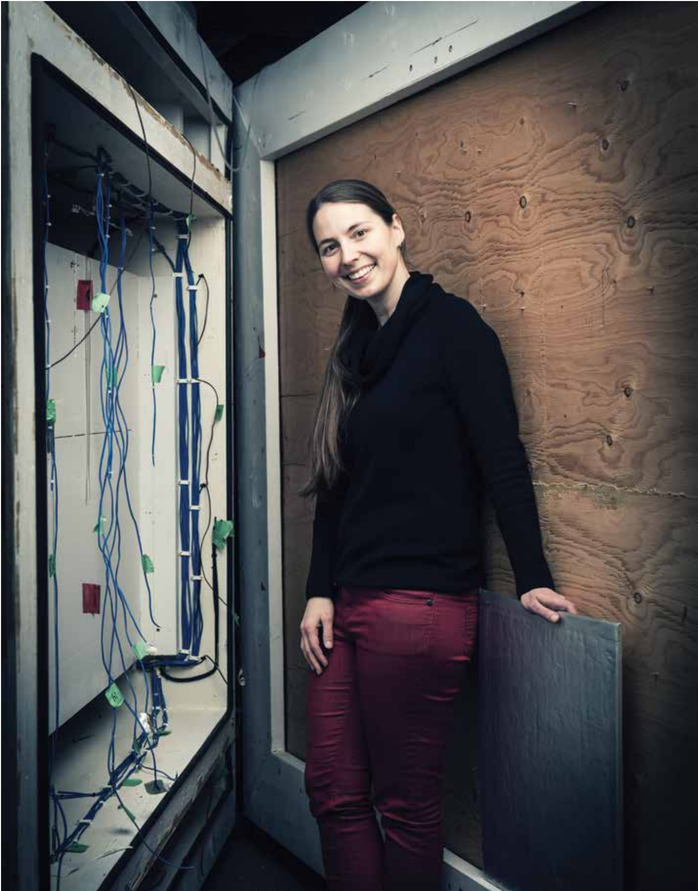
Cruickshank stands inside a guarded hot box, which she and her students use to determine the ability of a wall to resist the transfer of heat
