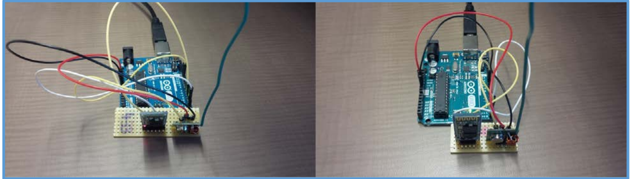
Figure 6: Final Circuit - Image of 434MHz (Left) Transmitter & 315MHz Transmitter (Right)
