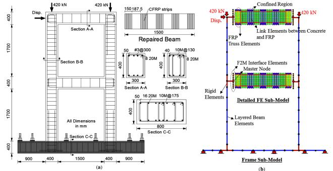
Fig. (4). (a) Details of the frame and repaired beam; (b) Mixed-type FE model of the frame.
