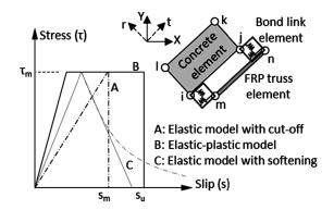
Fig. (2). FRP link element and different types of stress-strain relationship for bond.
