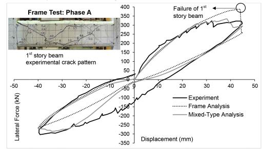
Fig. (5). Load-deflection response of the frame for Phase A.
