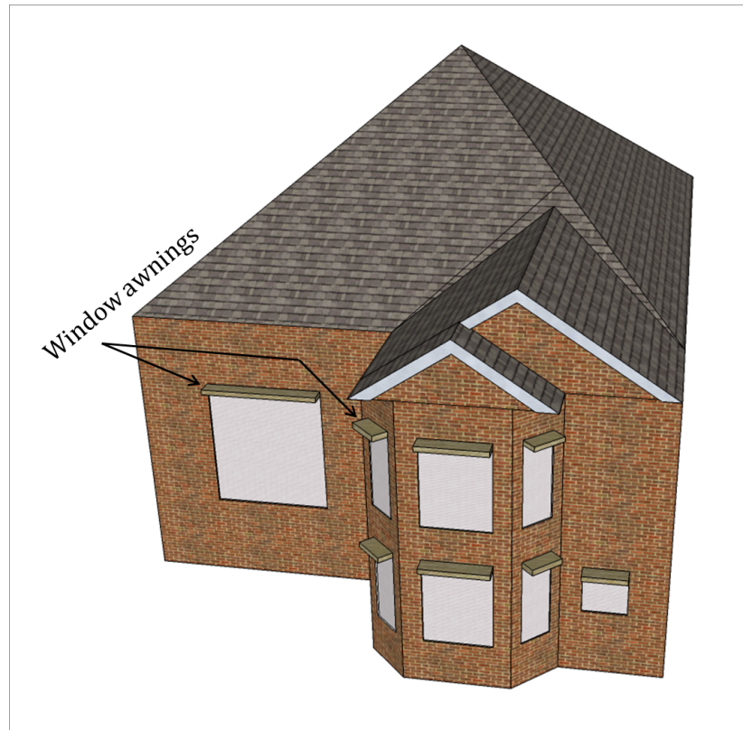
Figure 5.2: 30 cm window awnings on the south-west building face
