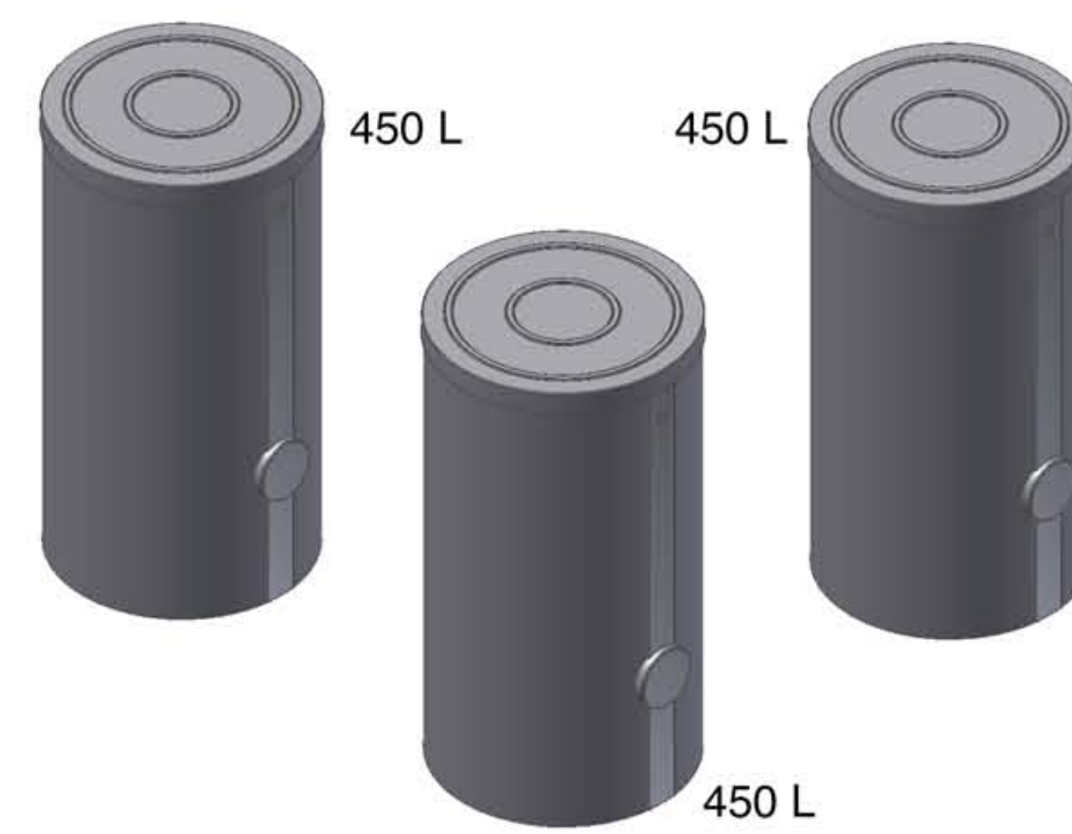
Water Store System 1 (Diurnal)
