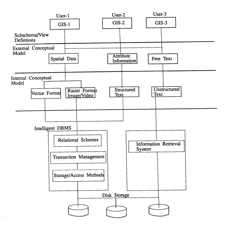
Figure 1: A typical GIS database architecture
