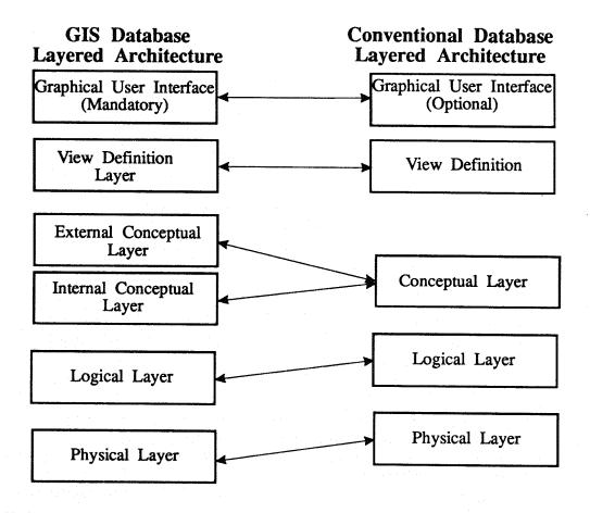
Figure 4: Correspondence between the levels of the proposed GIS and conventional database architectures
