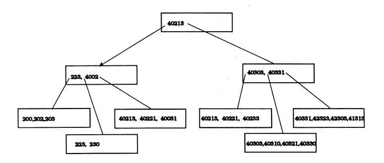
Figure 3: The  $B^+$ -tree index of order m = 5 for some quadcodes of Figure 2. In 32-bit representation, the first 4 bits store a level number.
