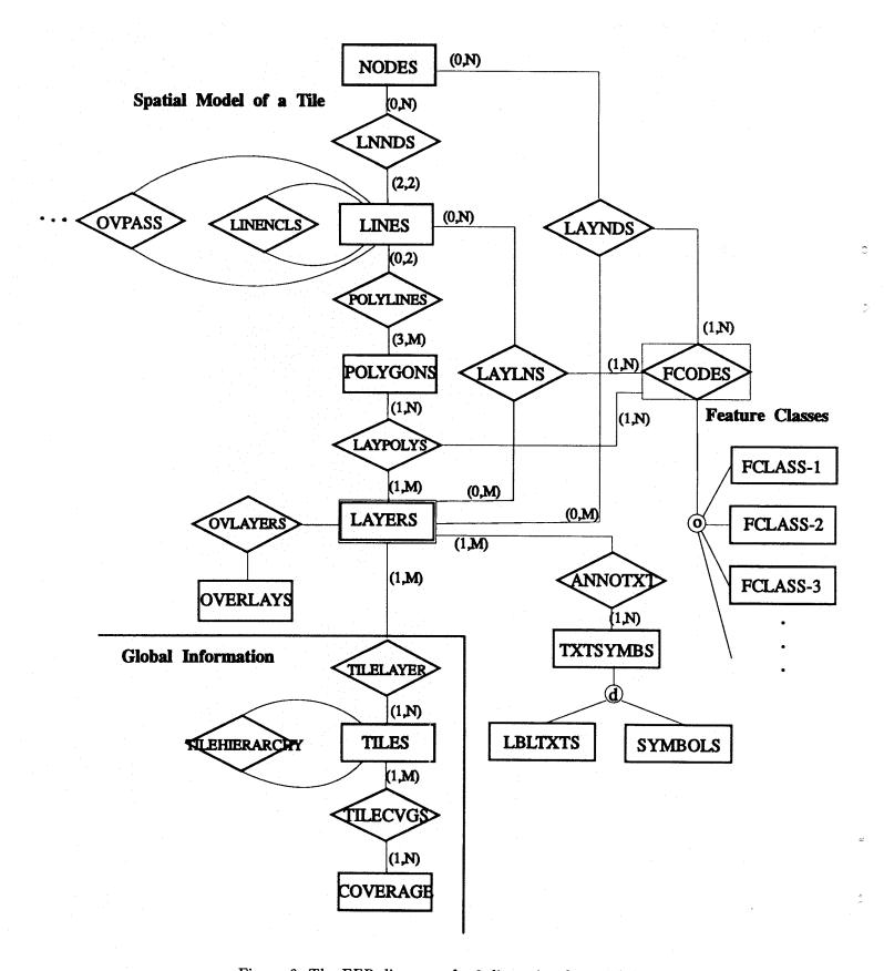
Figure 6: The EER-diagram of a 2-dimensional spatial data model
