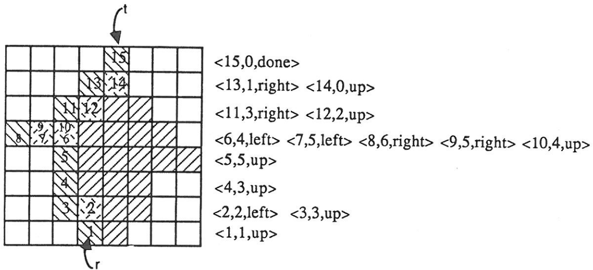
Figure 5: Encoding of a Rectilinearly Convex Robot's Inverted Image R'
