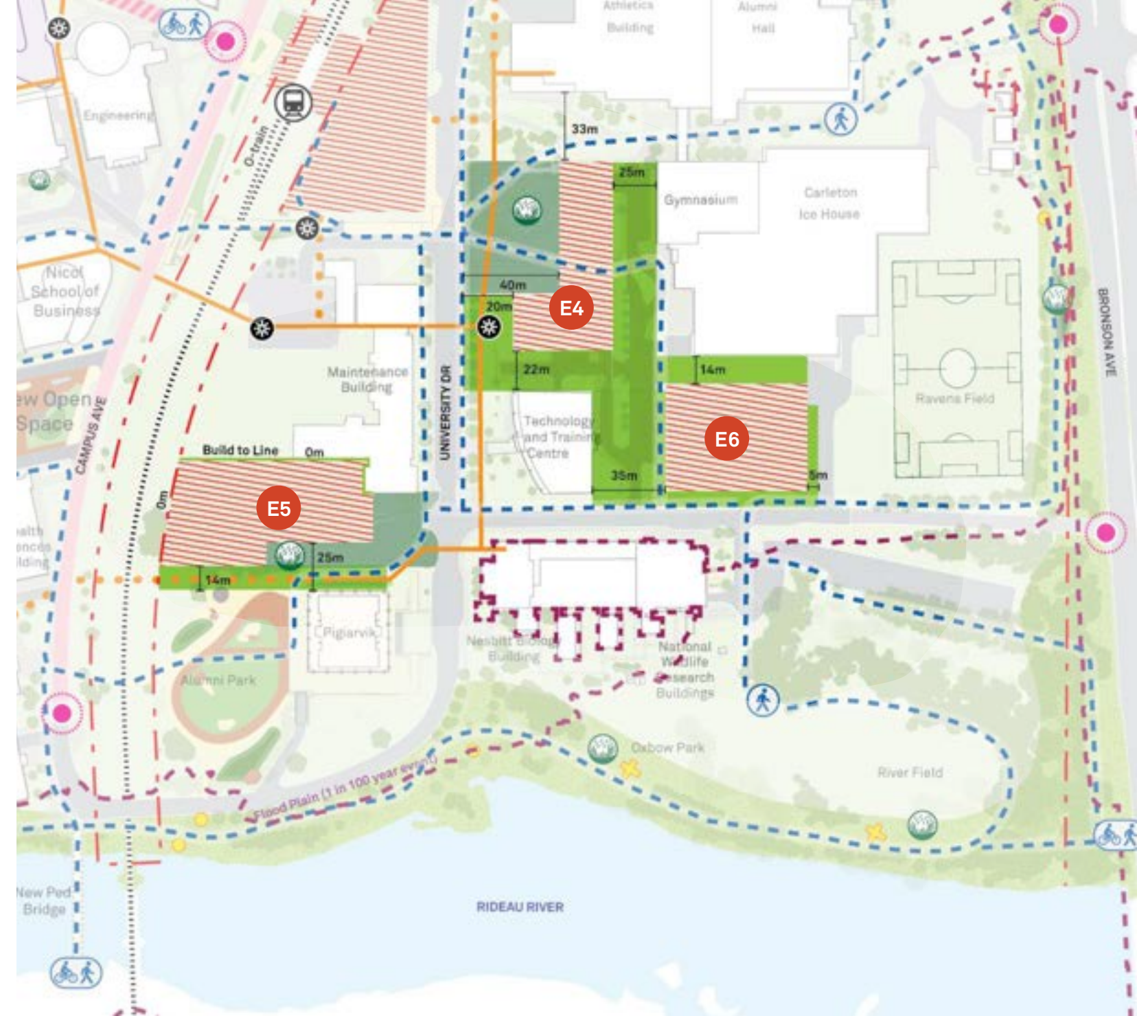
The above illustration shows Raven Road Sites ( E4-E6) potential buildable areas, setbacks, pedestrian connections, potential open spaces, and context.
