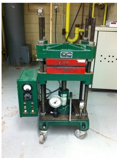
Figure 5.7: Heat press instrument for MEA fabrication
