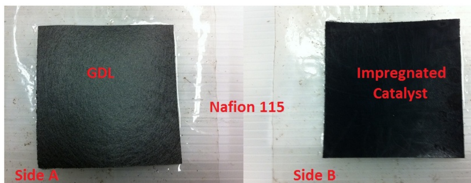
Figure 5.4: Membrane electrode assembly used in FE-DMFC stack
