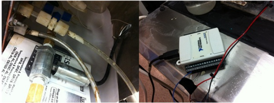
Figure 3.5: Views of differential pressure transducer (left) and DAQ card (right)
