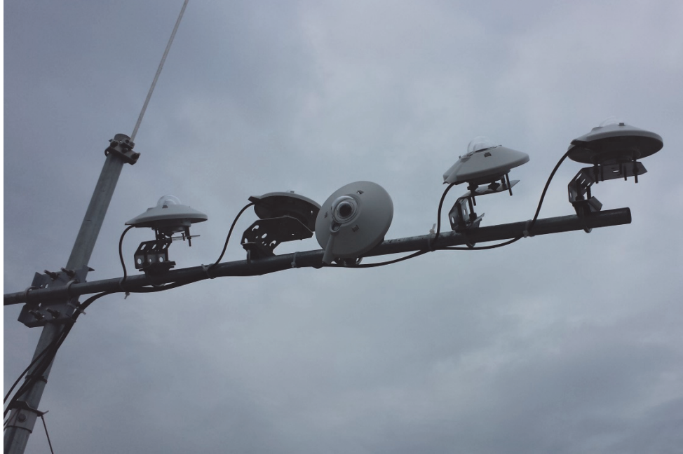
Figure A-2: Pyranometers installed (from left to right) at 30°, 0°, 90°, 45°, and 18°
