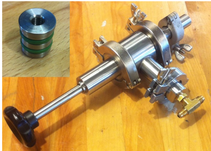
Figure 3-5: Adapter tool used for evacuation of sorption chiller and condenser plug (top left)
