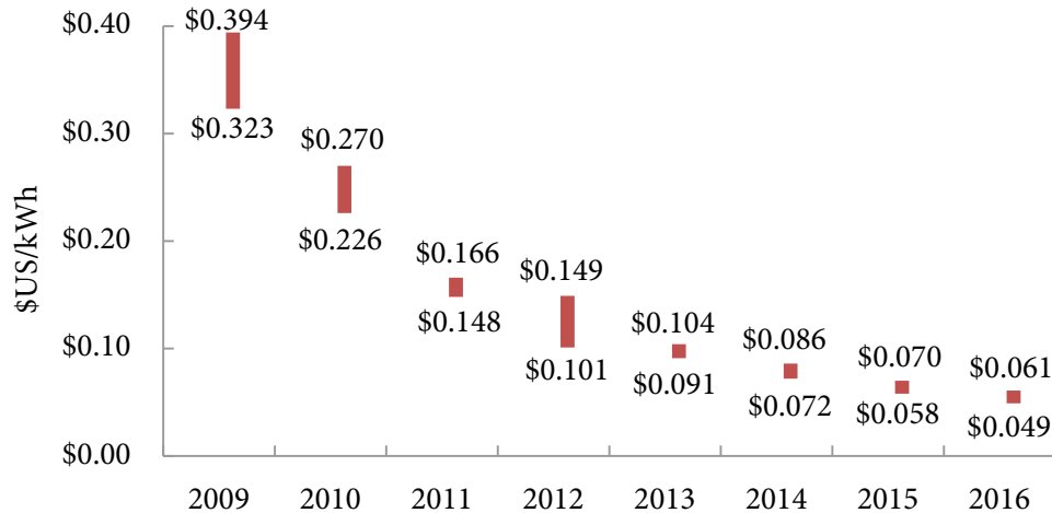
Figure B-1: Levelized cost of electricity of utility-scale solar PV power, contiguous United States
