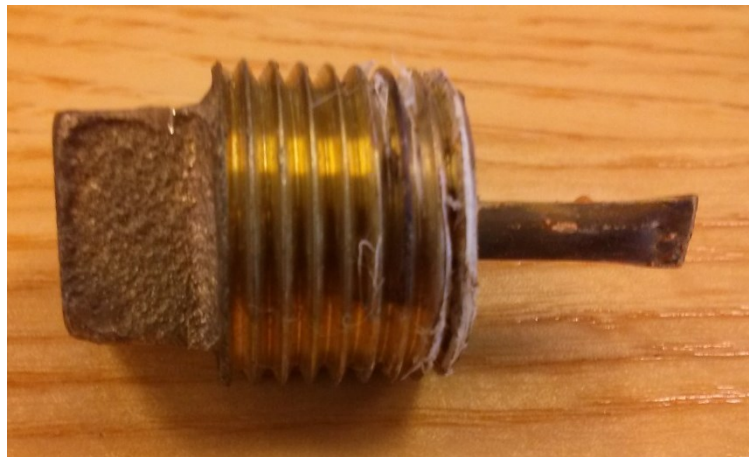
Figure 3-8: Custom Thermowell for Fluid Stream Temperature Measurement
