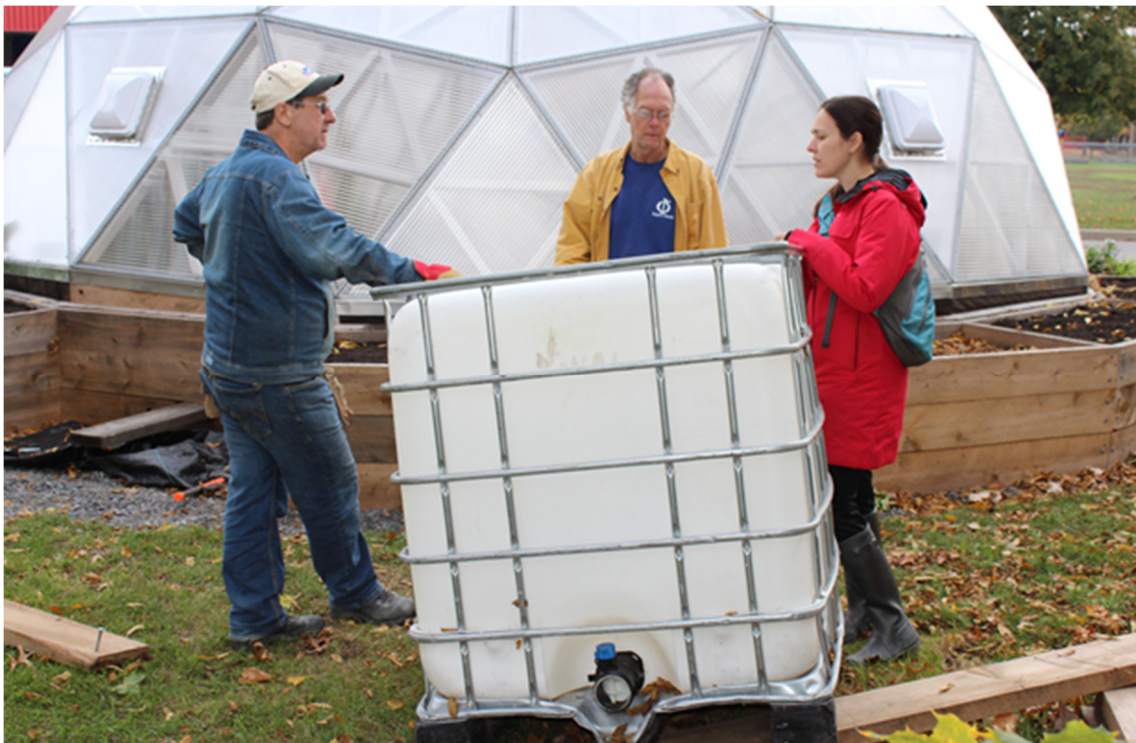
Figure 21: Intermediate bulk container to be used as a water storage tank (E. Kucerak, personal photograph, October 25, 2014). Adapted with permission.
