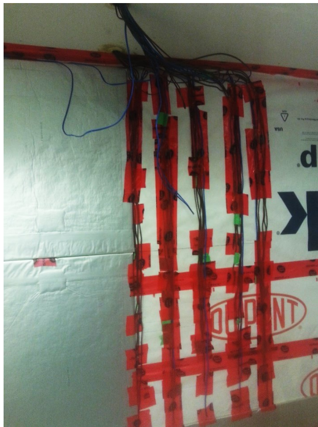
Figure 5-3: Thermocouple layout behind a single VIP with thermocouples
