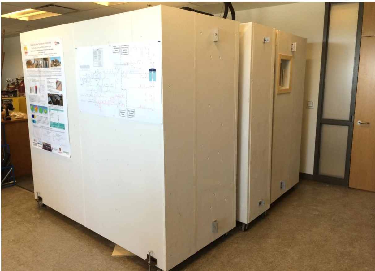
Figure 3-2: Photo of guarded hot-box located at Carleton University
