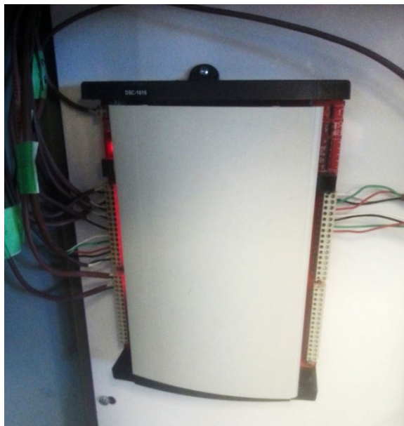
Figure 3-7: Photo of Delta controller integrated with the guarded hot-box
