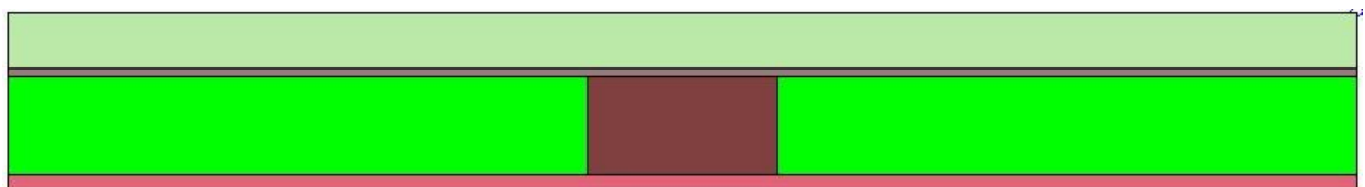
Figure 4-3: Simplified geometry of a code-built building envelope using a fictitious stud size in THERM
