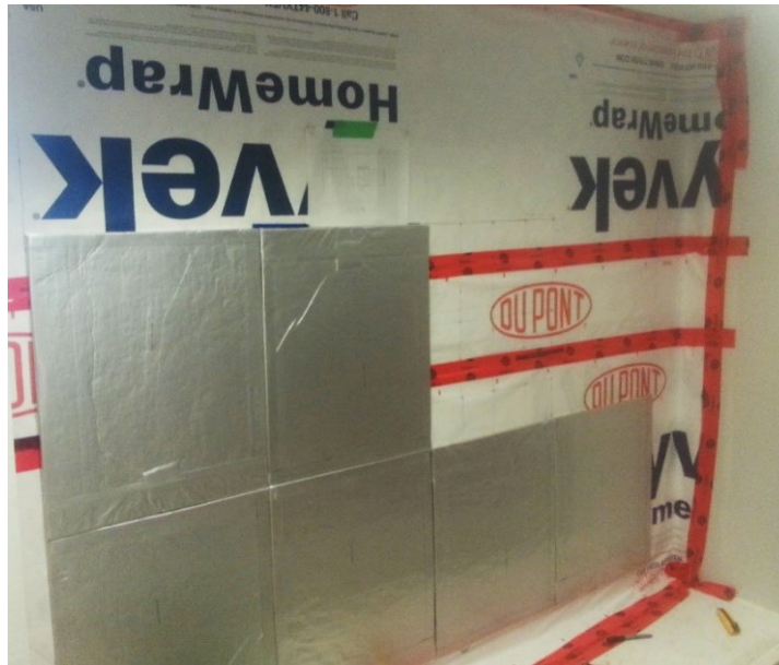
Figure 5-1: Single layer VIP configuration inside guarded hot-box
