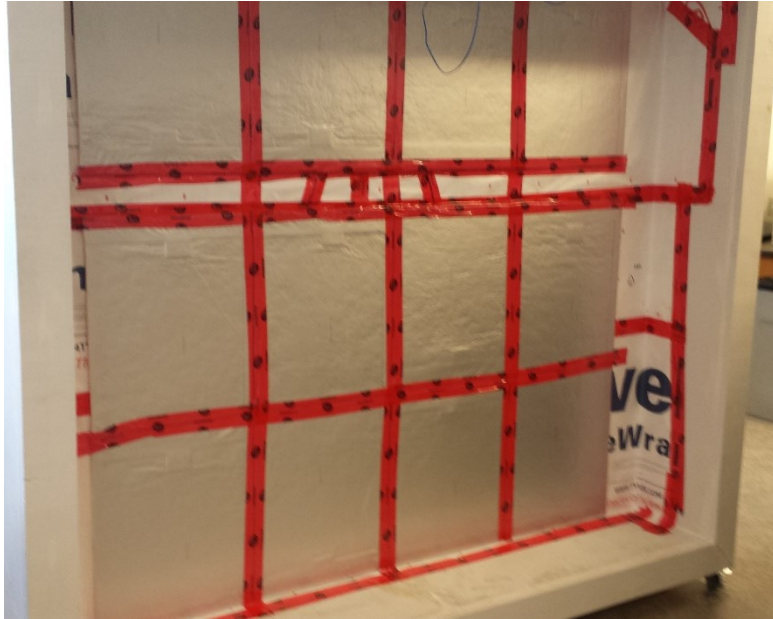
Figure 1-3: VIP installed on a building envelope in preparation for the guarded hot-box
