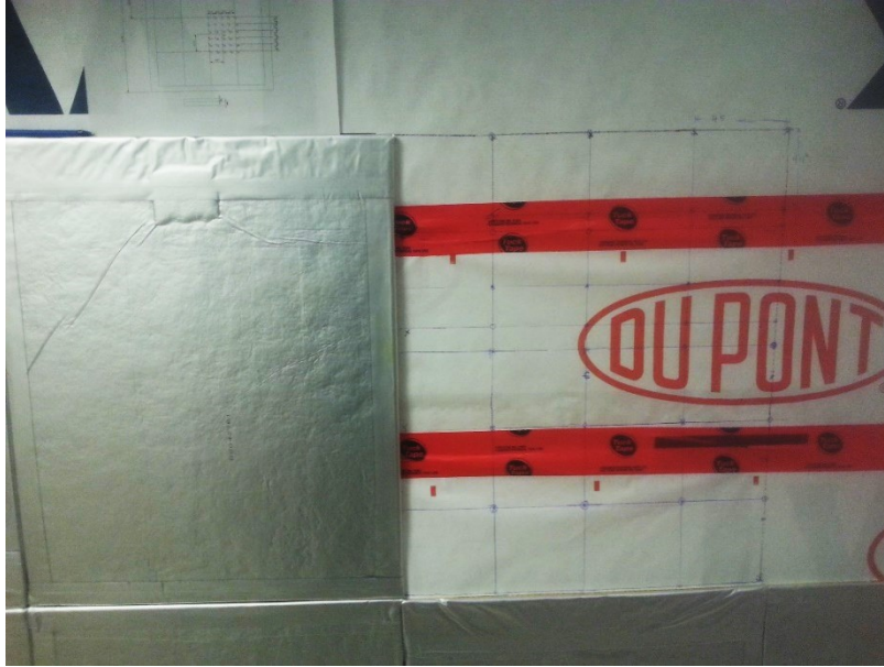
Figure 5-2: Thermocouple layout behind a single VIP without thermocouples
