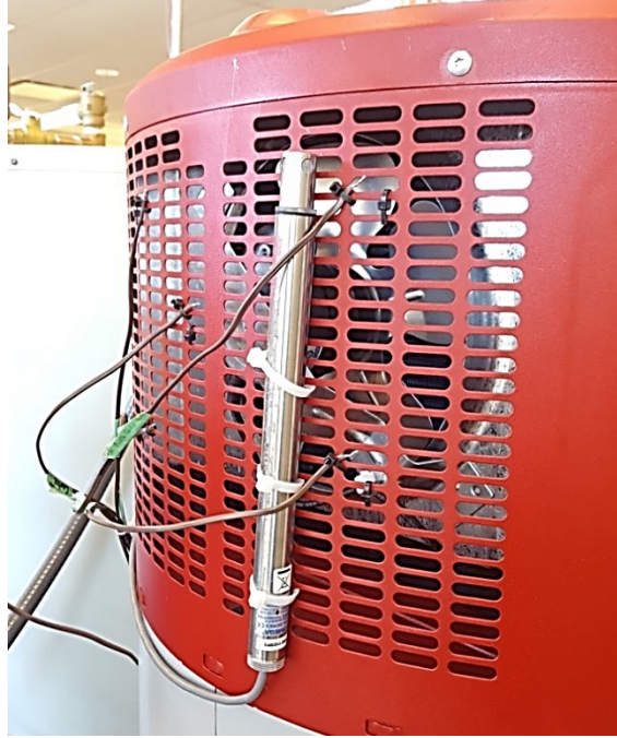
Figure 3-7: Heat pump water heater air exhaust instrumentation showing the “X” placement of the thermocouples and the RH sensor
