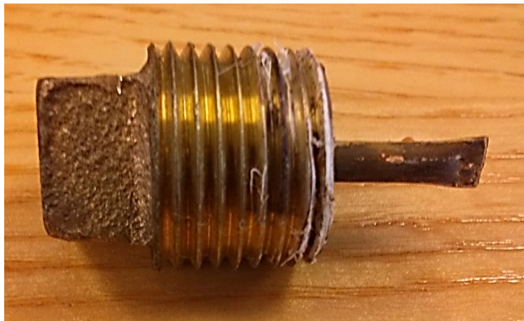
Figure 3-15: Thermowell for fluid stream temperature measurements
