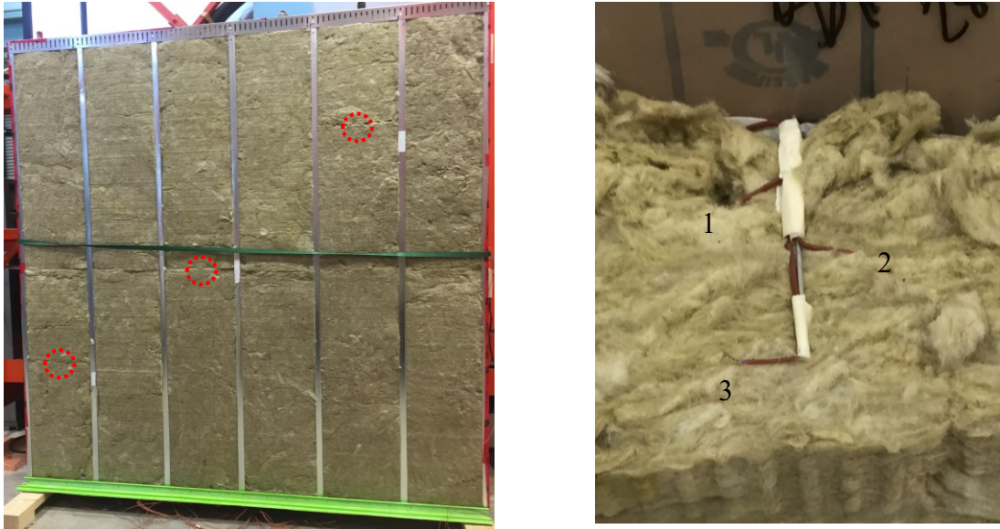
Figure 15: Thermocouple locations in the mineral fibre insulation. The red circle in the left photo indicates the instrumentation locations for the thermocouples at the centre of the stud cavities, through the depth of the mineral fibre insulation. The photo on the right is a close-up top view of the thermocouples through the depth of the mineral fibre at each location, located at 1in, 2in and 3 in from the gypsum board.
