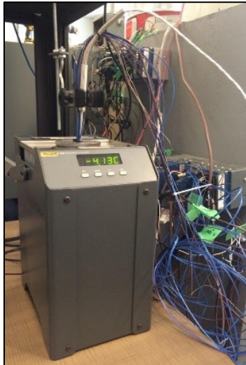
Figure A.14 Fluke 7102 Temperature Bath with Inserted RTD and Thermocouples
