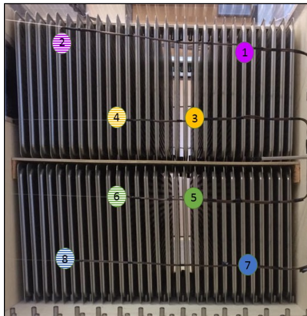
Figure 3.11 Temperature Measurement Positions at both the Inlet and Outlet of the PCM Storage Area
