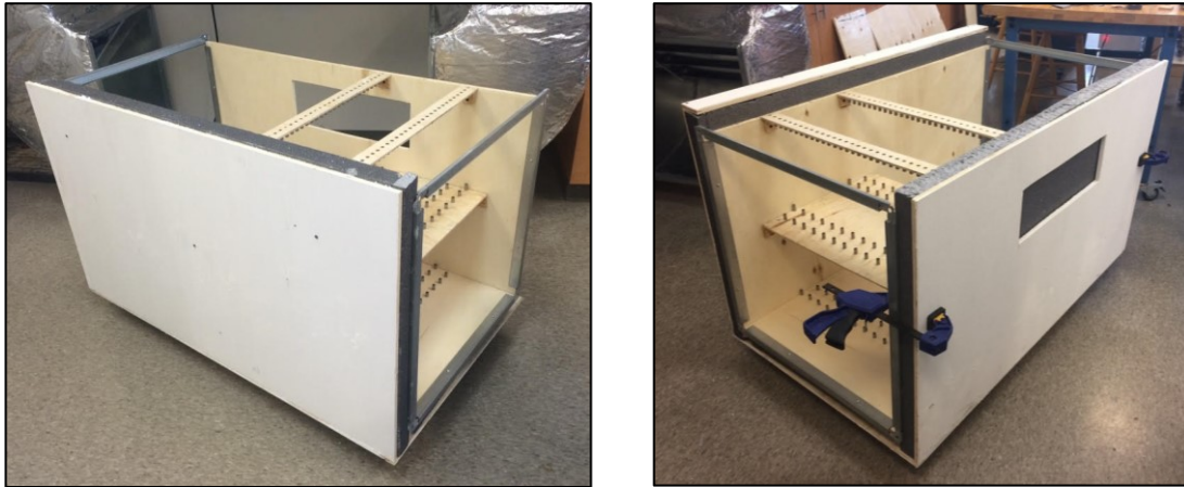
Figure A.7 Left) Side Wall Installed Right) Side Wall with Window Set in Place with Small Clamps
