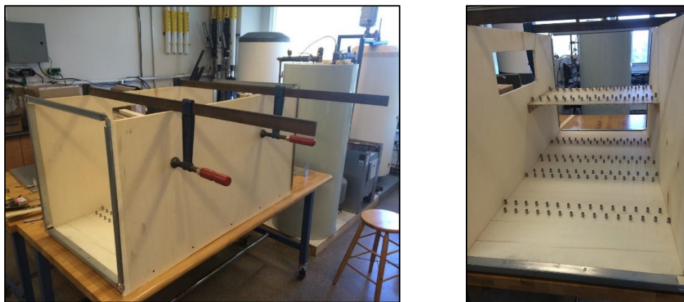
Figure A.4 Left) Large Clamps on Inner Box Walls and Right) Middle Plate Installed
