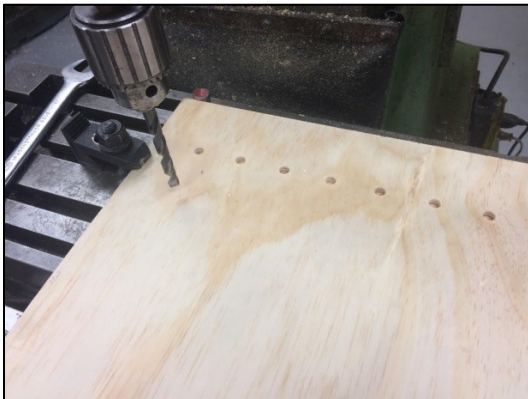
Figure A.1 Left) Holes being Drilled into the Middle Plate and Right) Holes being Drilled into the Top Bars
