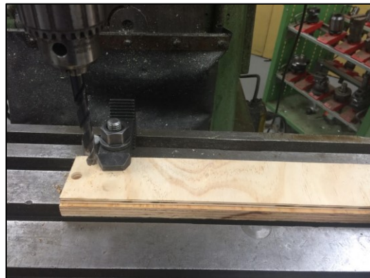
Figure A.1 Left) Holes being Drilled into the Middle Plate and Right) Holes being Drilled into the Top Bars
