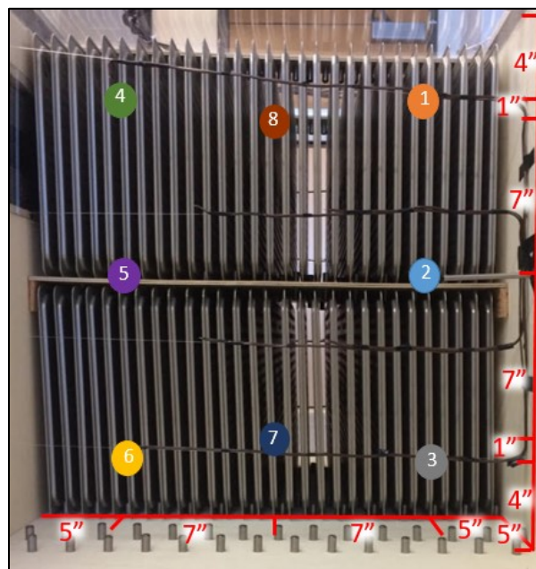
Figure 4.2 Velocity Sensor Locations of First Velocity Profile Configuration
