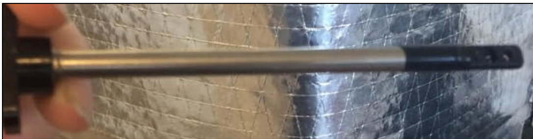
Figure 3.12 Cambridge Accusense F900 Series Air Velocity Sensor
