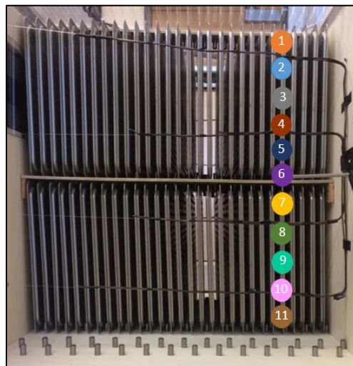
Figure 4.4 Velocity Sensor Locations of Second Velocity Profile Configuration
