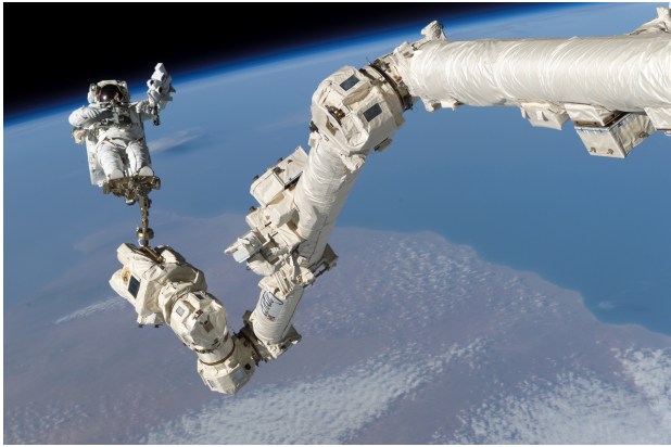
Figure 3: Canadarm2 on-board the ISS that assists with maintenance, docking, capturing payloads and EVAs (credit: NASA STS-114 Shuttle Mission Imagery)
