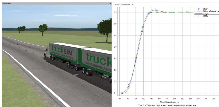
Figure 5 Sample output of transient high-speed off-tracking in a high-speed lane change maneuver
