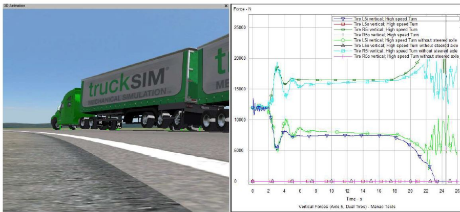
Figure 8 Output sample of static rollover threshold from the high-speed turn with increasing curvature maneuver
