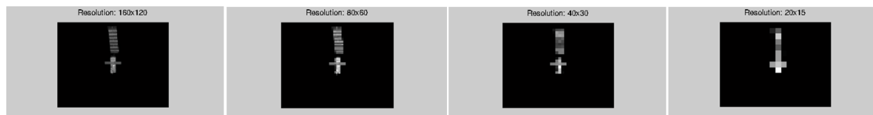
Figure 11. Reduction in image resolution using pyramids
