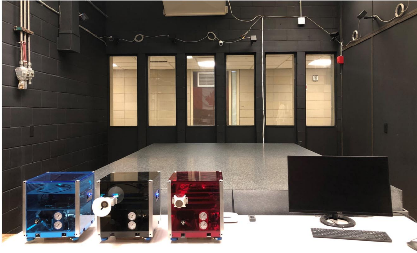
Fig. 8 The spacecraft proximity operations testbed.
