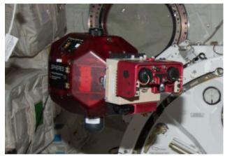
Fig. 3 SPHERES satellite equipped with the VERTIGO Goggles operating onboard the ISS.
