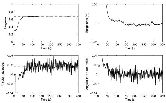
Fig. 10 Range to target spacecraft and angular velocity of the inspector spacecraft.
