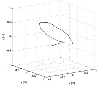
Fig. 12 On-orbit experimental results: 3-D visualization of the inspector spacecraft circumnavigation trajectory.
