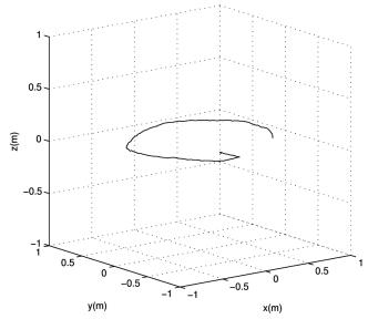
Fig. 8 Simulation results: 3-D visualization of the inspector spacecraft circumnavigation trajectory.
