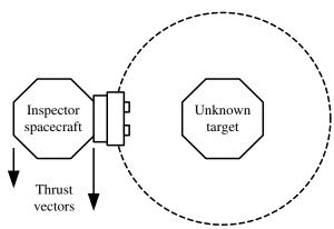
Fig. 4 Different thrust requirements to circumnavigate around a target, considering an offset c.m.
