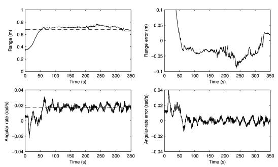
Fig. 14 On-orbit experimental results: range to target and angular velocity of inspector spacecraft.
