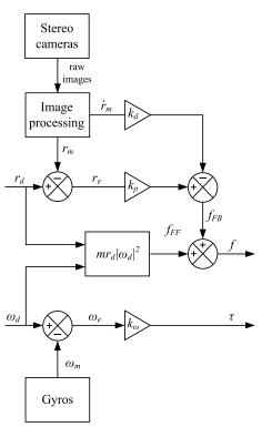
Fig. 1 Vision-based control strategy block-scheme implementation diagram.
