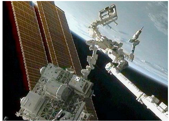
Fig. 4. Canadarm2 and Dextre performing a demo of a robotic refueling task [35].
