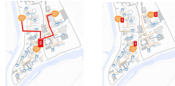
Figure 47 - (Left) Central TES with connection to each nodal plant, (Right) TES Tank at each nodal plant (TES Tanks are shown are for visualization purposes and do not represent required tank sizes. Distribution pipe routing shown is also indicative)
