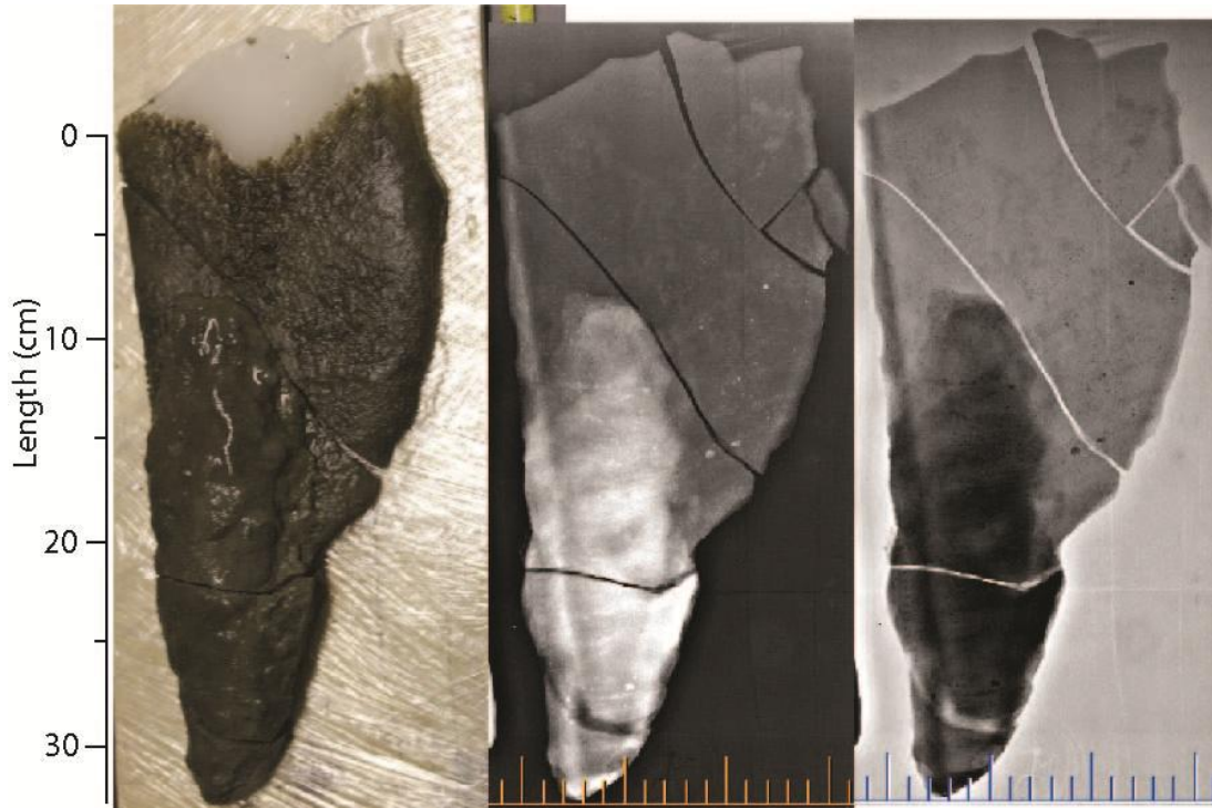
Figure C16. Freeze core ROAD10-46-1, Face 1 of 2, Section 1 of 1: (left) light photograph; (middle) positive X-Ray; (right) negative X-Ray. The big bars on the X-Ray scale are separated by 5 cm and the small bars are separated by 1 cm.
