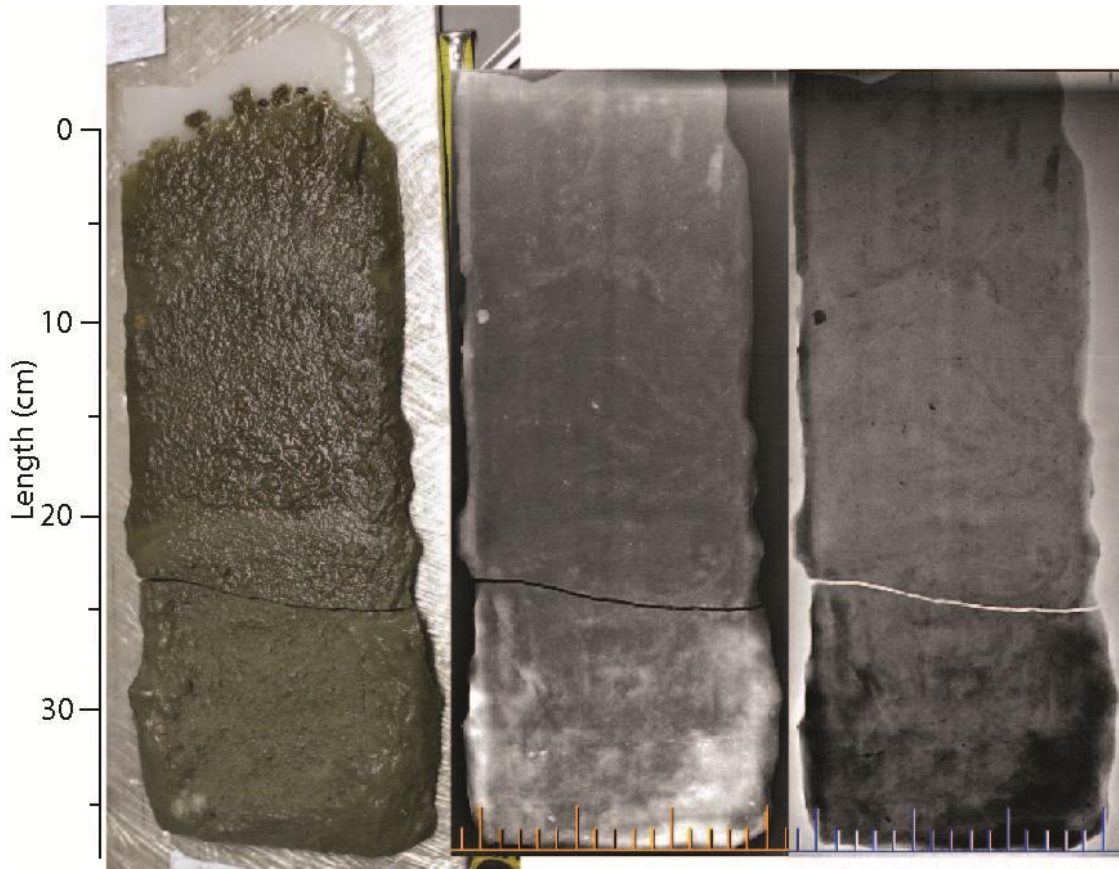
Figure C17. Freeze core ROAD10-46-1, Face 2 of 2, Section 1 of 1: (left) light photograph; (middle) positive X-Ray; (right) negative X-Ray. The big bars on the X-Ray scale are separated by 5 cm and the small bars are separated by 1 cm.
