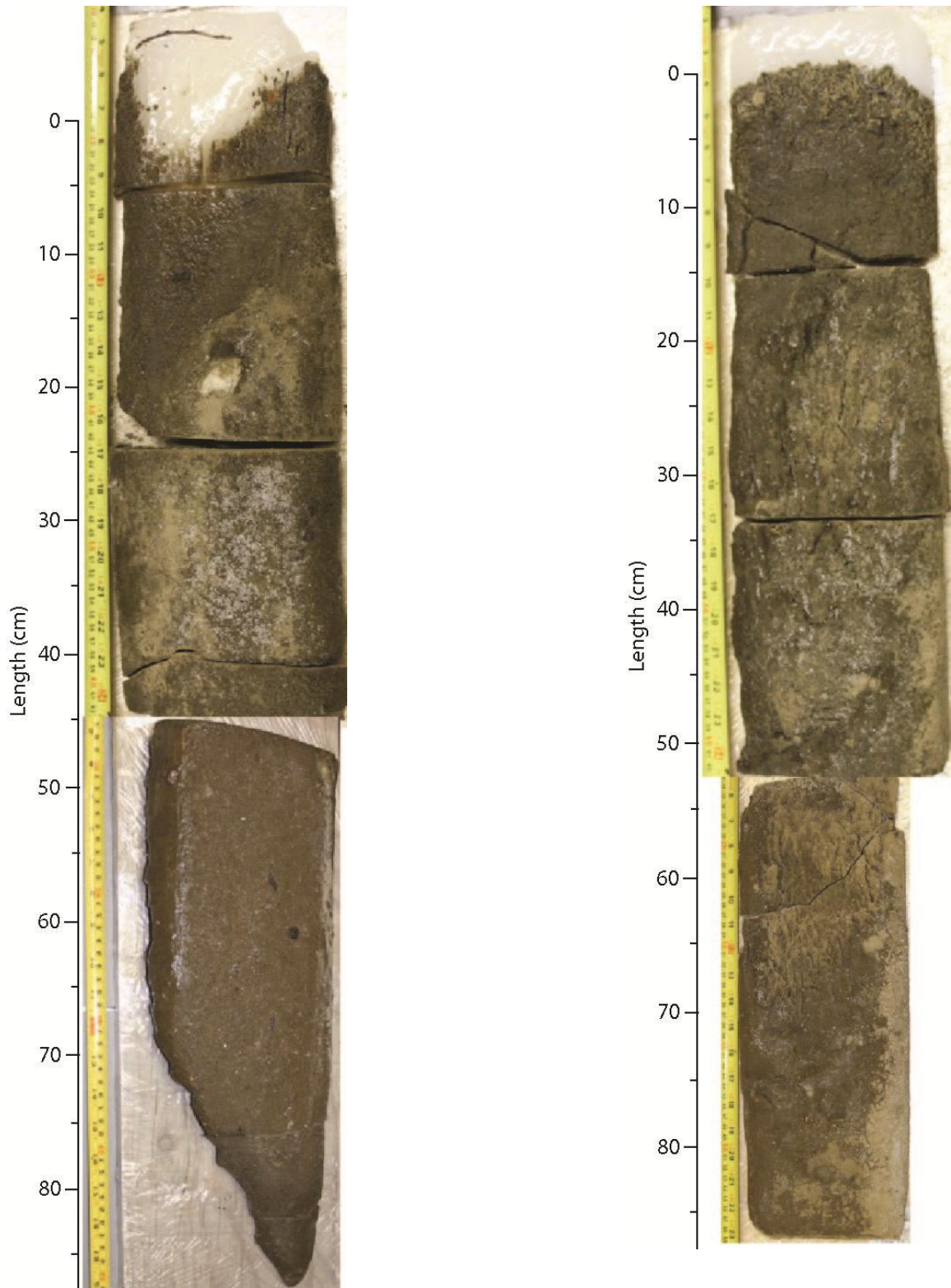
Figure C25. Freeze core ROAD10-ECHO, Face 1 of 2, Sections 1 & 2: (left) light photograph of Section 1; (right) light photograph of Section 2.
