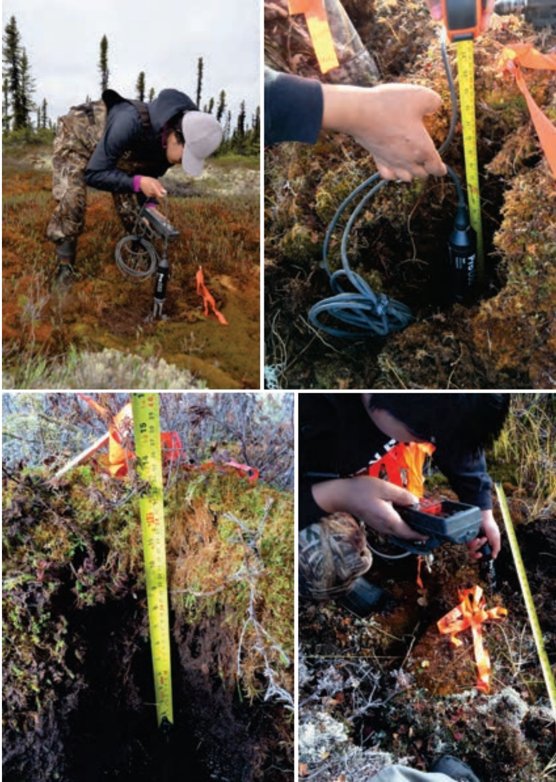
Figure 18: Julienne Chipesia (top left) and Charlie Snowshoe Jr (top right, bottom) measuring water table depth, pH, and specific conductivity. Photo credits: S. Lord, GRRB, 2020.
