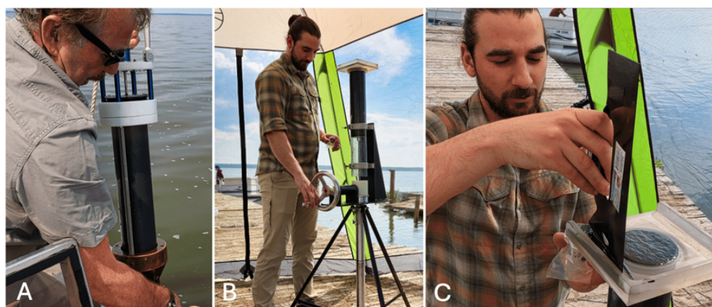
Figure 2. Photographs showing (A) collection of a UWITEC gravity core from Utikuma Lake as the bottom of the core is capped upon recovery, (B) a UWITEC core barrel filled with a core mounted on a custom-built portable extruder that can be deployed in the field and which can produce 1 mm resolution subsamples, and (C) a 1 mm resolution subsample being transferred from the extruder into a sample bag for subsequent analysis.
