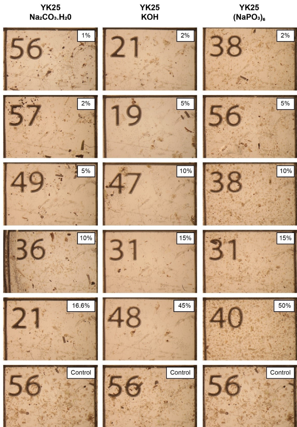
Figure 2. 4: Photomicrographs showing the level of organic content reduction in chemically treated, with different concentrations of soda ash, KOH, and Calgon, and control YK25 sub-samples.
