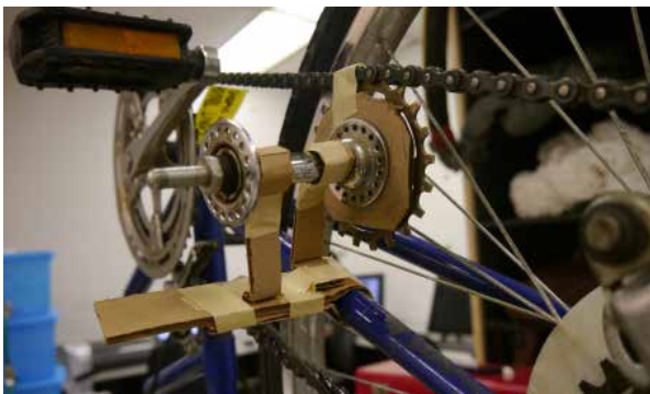
Engaging sprocket to the chain
