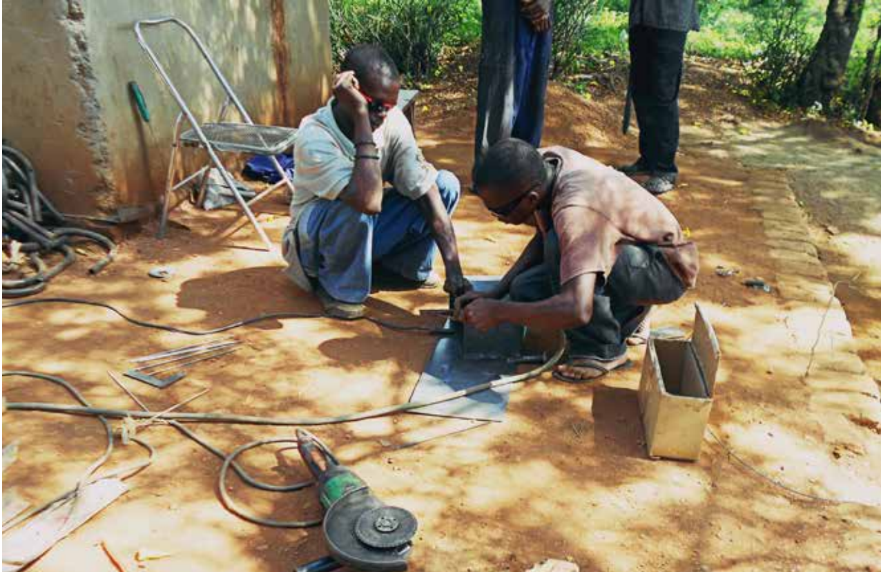
At the workshop, Kio's helpers cut and weld sheet metal together for a prototype.
