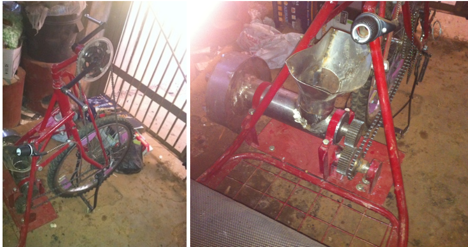
Figure 21. Re-engineered Local Made Peanut Grinder Mechanism (Perez Magoola)
