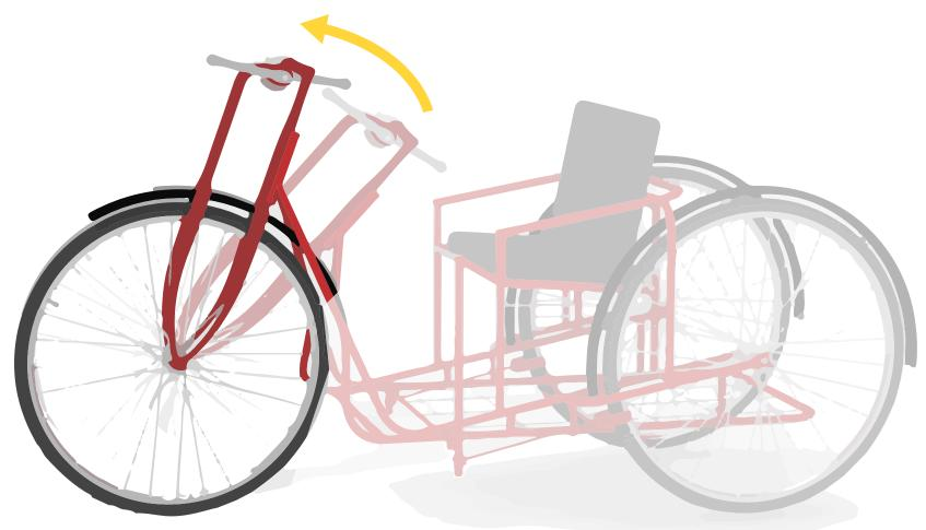
Increasing the angle of the steering column will reduce the risk of the load of the tricycle deforming the wheel.
