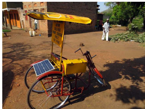
Figure 3: Tricycle with solar-charging attachment for cell phones, designed by Andrew Theobald (Harambee Uganda Project, 2013).
