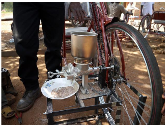
Figure 2: Tricycle with ground nut grinding attachment, designed by Carmen Liu (Harambee Uganda Project, 2013).
